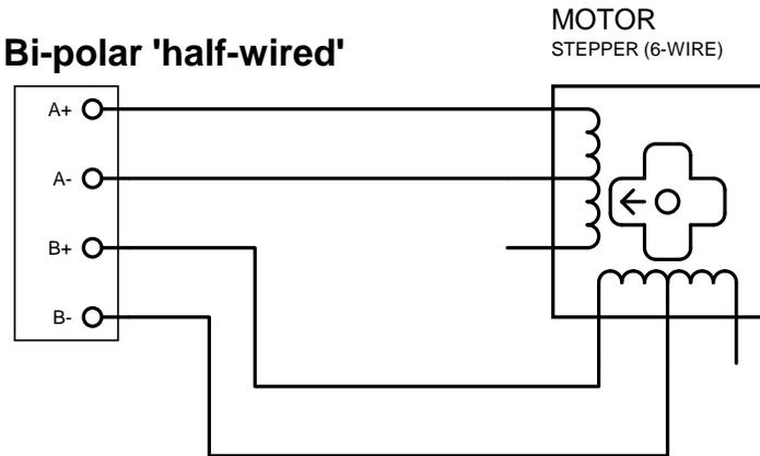
One pole of each winding and the centre tap are connected the other pole of each winding should be taped off and isolated.
